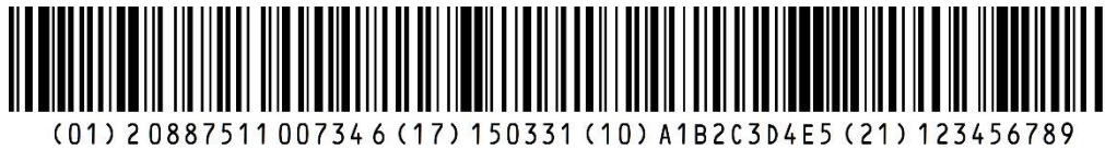
Figure 6-1 GS1-128 - linear barcode
