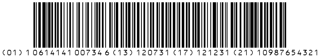
Figure 5. Sample GS1-128 barcode with GTIN (01), Packaging Date (13), Expiration Date (17), and Serial Number (21)
