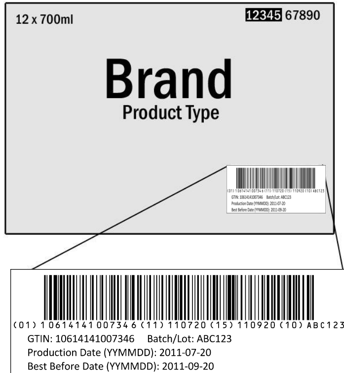
Figure 17. Sample case label showing use of GS1-128 barcode and human-readable text to communicate GTIN (01), Batch/Lot Number (10), Production Date (11) and Best Before Date (15)
