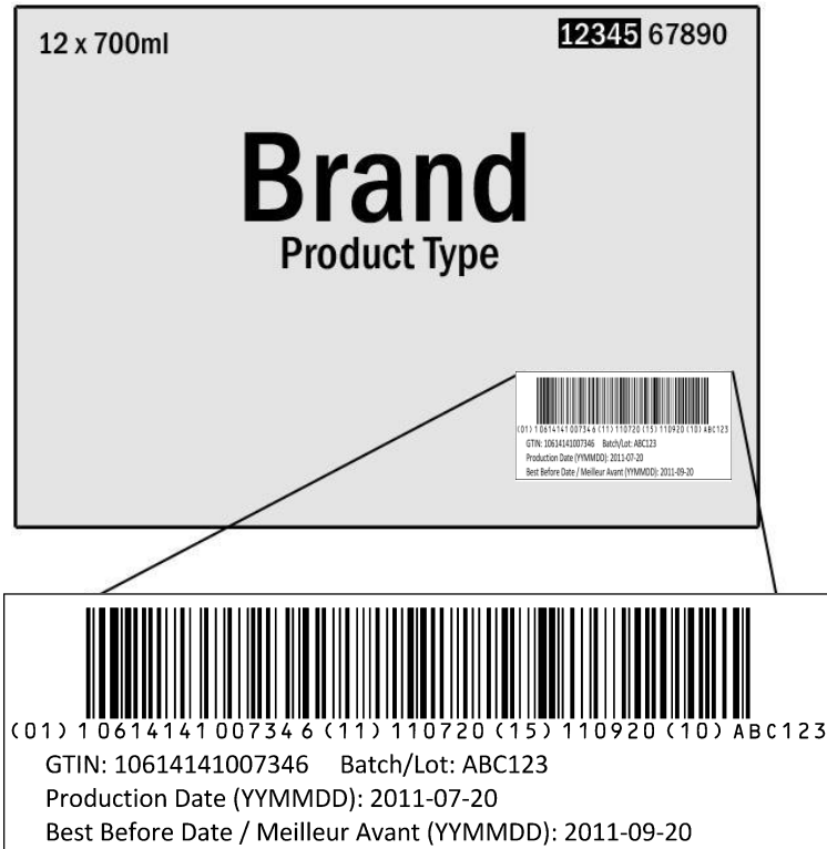
Figure 18. Sample case label showing use of GS1-128 barcode and human-readable text to communicate GTIN (01), Batch/Lot Number (10), Production Date (11) and Best Before Date (15) as well as both English and French translations which are required when distributing to Canada
