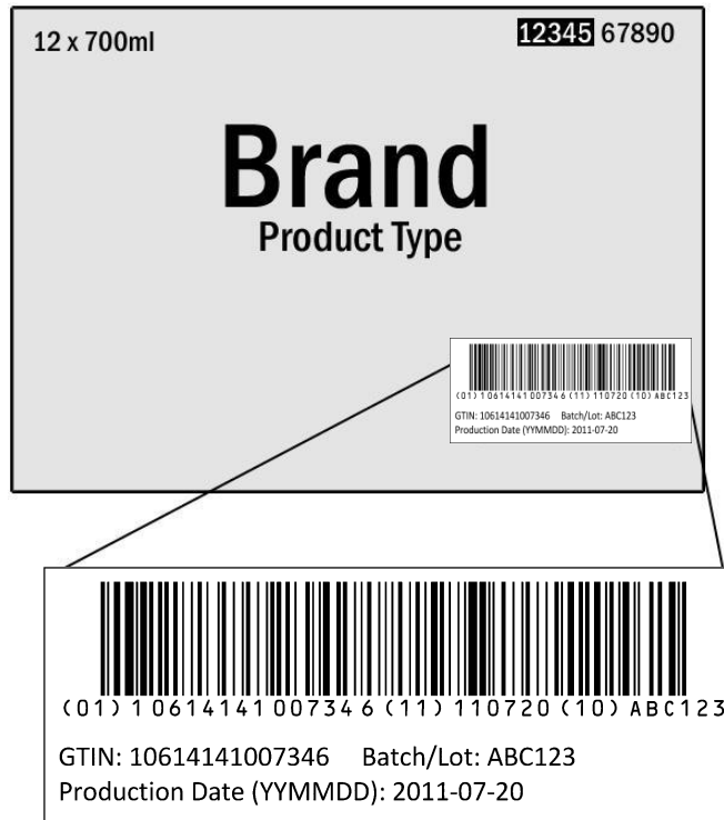
Figure 16. Sample case label showing use of GS1-128 barcode and human-readable text to communicate GTIN (01), Batch/Lot Number (10) and Production Date (11)
