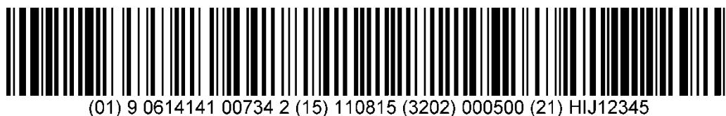
Figure 6. Sample GS1-128 barcode with GTIN (01), Best Before Date (15), Net Weight (3202), Serial Number (21)
